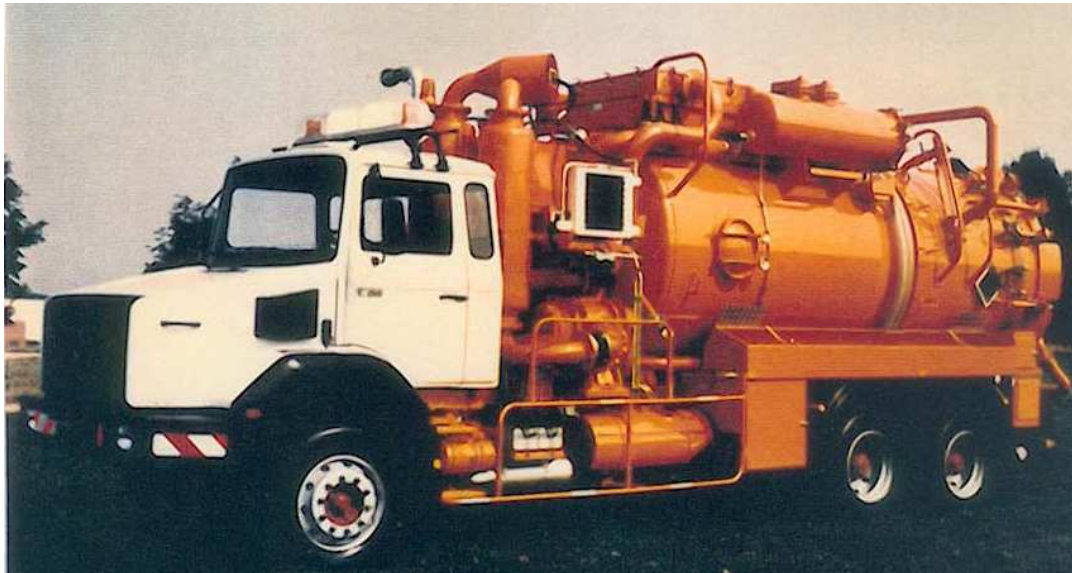
Positive displacement blower Hibon, air injection series, installed on a vacuum truck for sewage cleaning. Installation : FRANCE.
